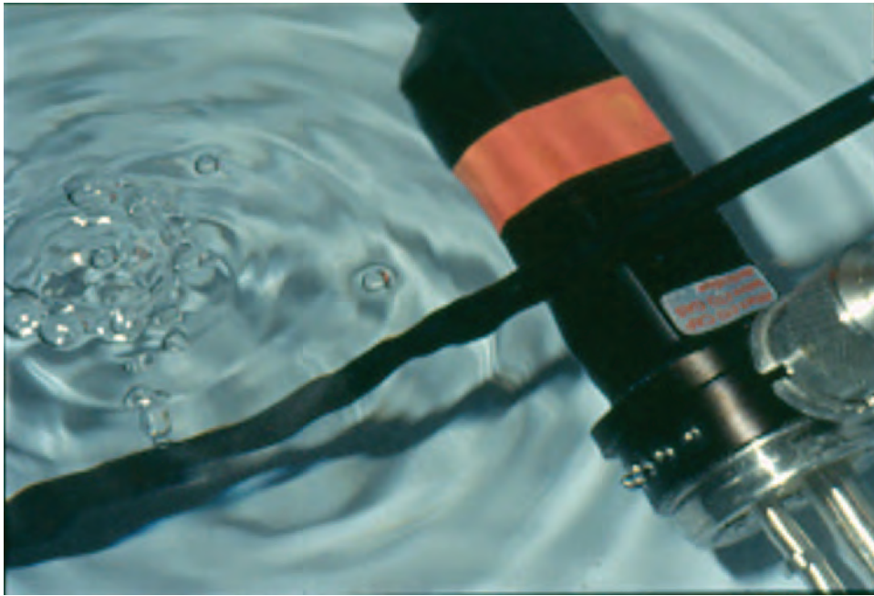
FIGURE 4. Positive leak test result. Air bubbles emitting from the surface of the bronchoscope indicate a breach in its exterior.
